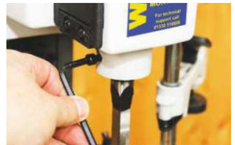
▲ You need a hex wrench to secure the chisel
